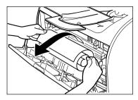
If the leading edge of the paper has already entered the imaging area, gently pull out the paper at the face up paper output rollers until the edge of the paper appears.
